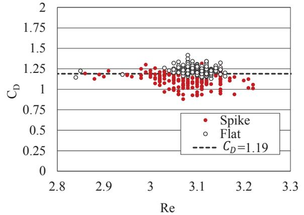
**(a) Around 3m/s (Re=1985)**
