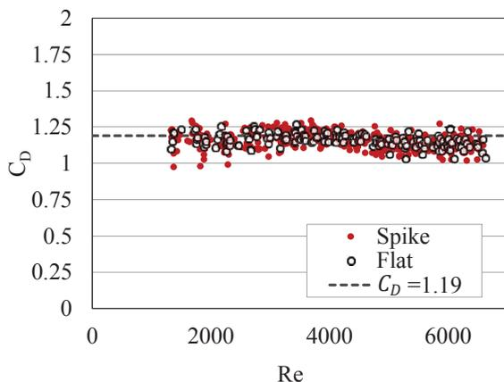
**Fig. 6 Drag coefficient at each Reynolds number**
