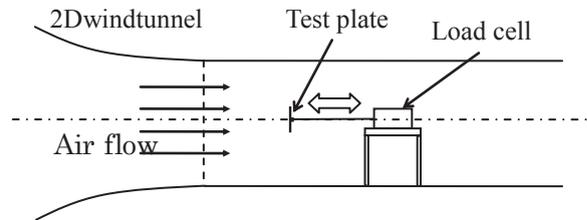
**Fig. 4 Experimental set-up of drag force measurement**
