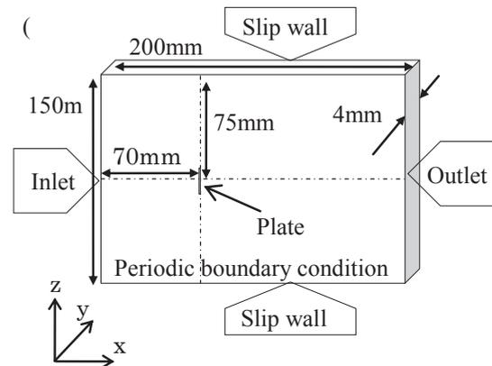
**Fig. 5 Boundary condition for analysis**
