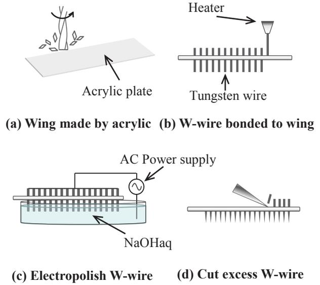
**Fig. 2** Fabrication method of the artificial wing having spikes
