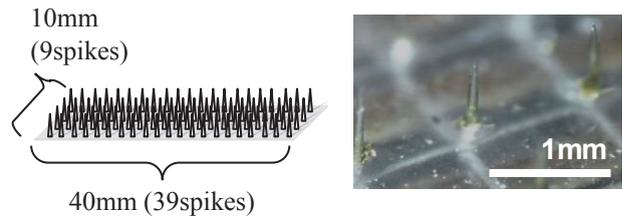
**Fig. 3 Overview of artificial spike plate**
