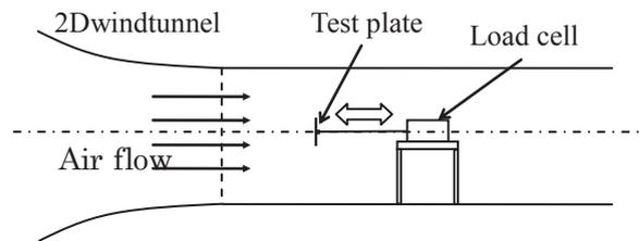
**Fig. 4** Experimental set-up of drag force measurement
