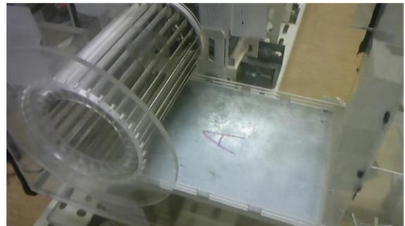
**Fig. 8 Impeller and tongue used in experiment**
