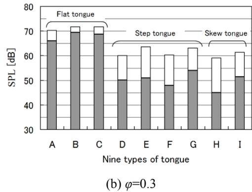
**Fig. 7 Overall noise level and rotation noise level for 9 types of tongue**
