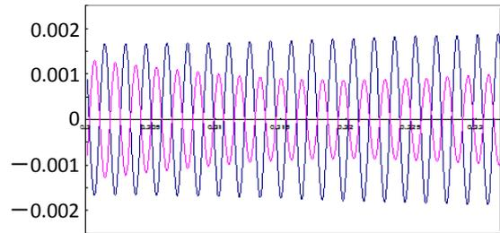
**Fig. 12** Comparison of pressure waves for mounting point 1/4 and 3/4 of stepped tongue E
