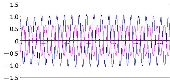
**Fig. 13** Comparison of velocity waves for mounting point 1/4 and 3/4 of stepped tongue E
