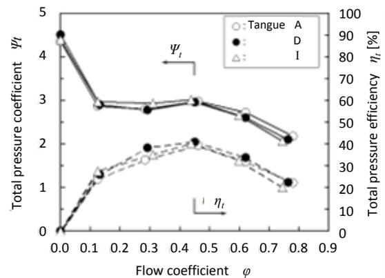
**Fig. 4 Relation between total pressure coefficient  $\psi_t$  and total pressure efficiency  $\eta_t$  for tongues A, D and I**
