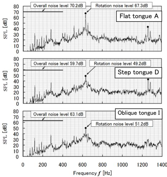
**Fig. 6 Comparison of spectra of acoustic signal for tongues A, D and I (low flow rate region for  $\varphi=0.3$ )**
