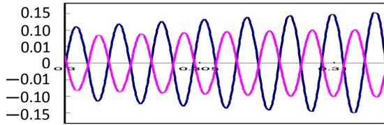
**Fig.15 Comparison of sound waves for mounting point 1/4 and 3/4 of oblique tongue H**
