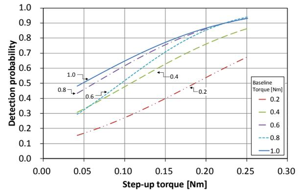
**Fig. 6 Fitting Curves of the Detection Probabilities (Target Angle: 45°).**
