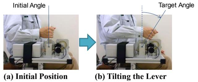
**Fig. 2 Trial of Manipulation with Resisting torque.**
