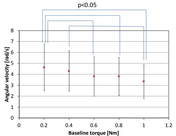
**Fig. 7 Angular Velocity of Lever at the Moment of Reaching to Target Angles**
