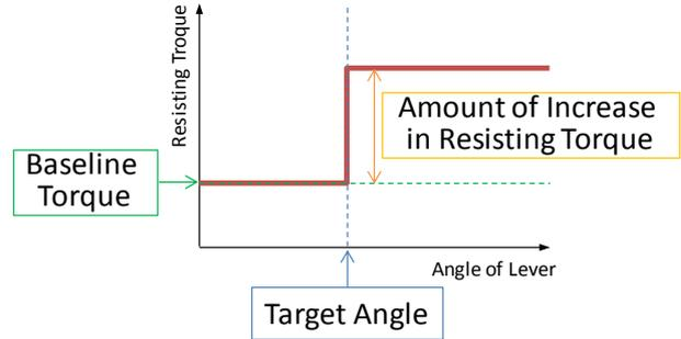
**Fig. 3 Change in Resisting Torque from Baseline Torque to Step-Up Torque around the Angle of Target.**
