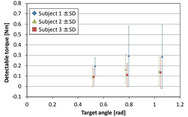
**Fig. 4 Minimum Noticeable Increase in the Resisting Torque at the Three Target Angles.**
