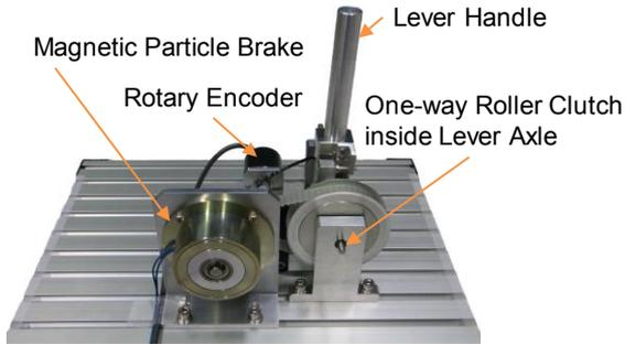
**Fig. 1 Manual control lever with Magnetic Brake that is Connected by One-way Clutch Mechanism.**
