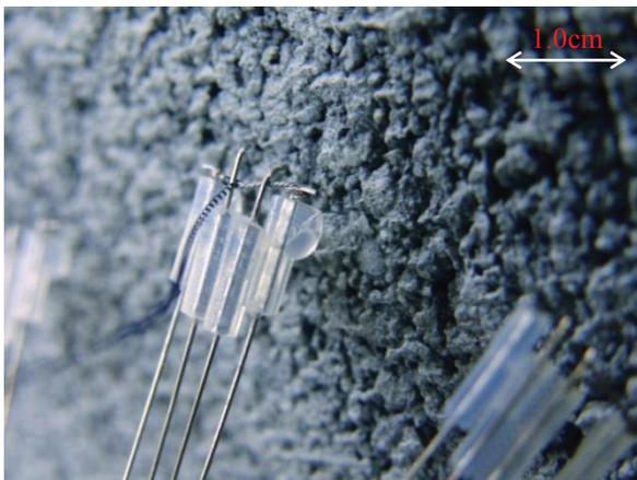
**Fig. 11 Surface of concrete wall and claw of the robot**
