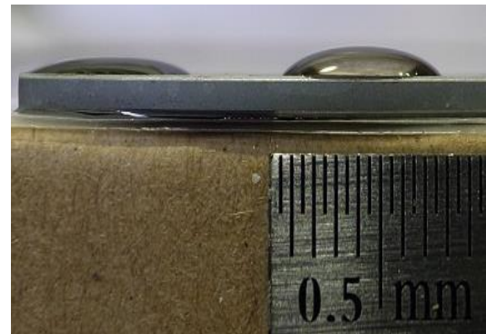
Fig.9 Measurement of wetting angle on piston ring
