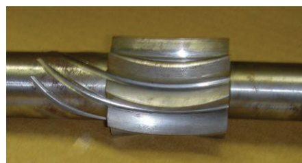
(a) Pinion with circular-arc tooth-trace
