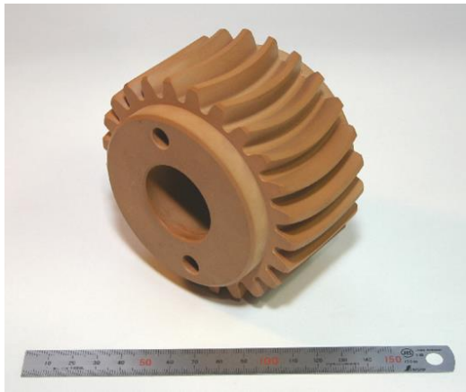
(b) Pinion ( m4, z=24, R=70mm )
