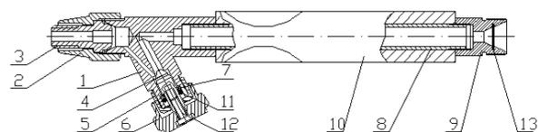
**Fig. 2** Gas burner structure
