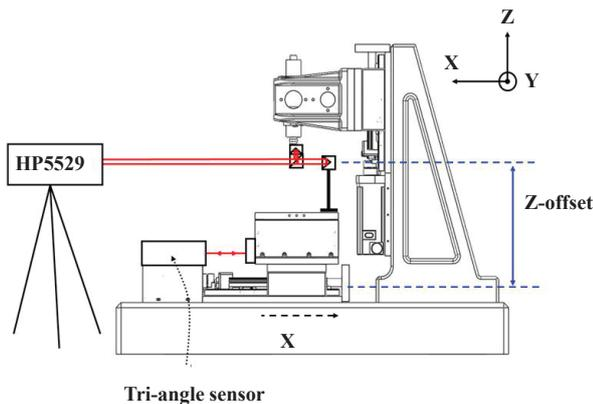
Fig. 8 Experimental setup for X-positioning test
