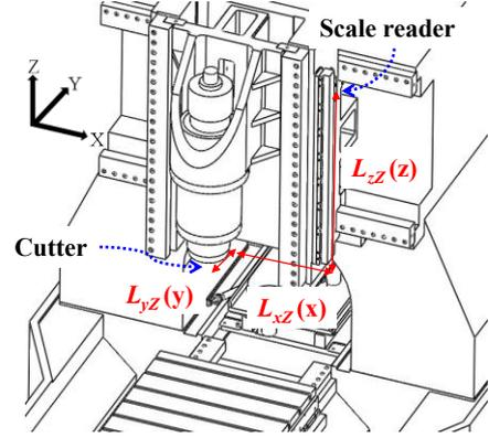
**Fig. 6** Abbé offset of Z-axis motion
