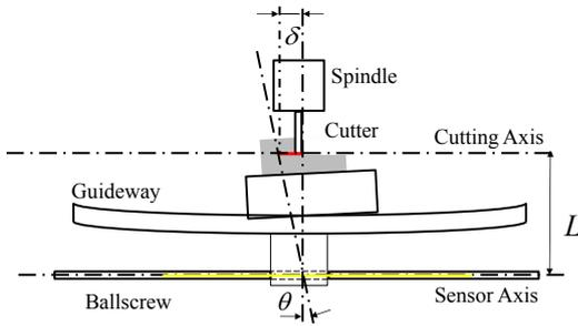
**Fig. 2 Cutting point error due to Abbé error**
