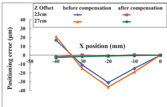
Fig. 9 Experimental results of X-positioning error calibration
